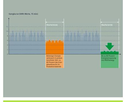
PROFIenergy significantly reduces the energy consumption during idle times, and allows intelligent energy management PROFIenergy:
