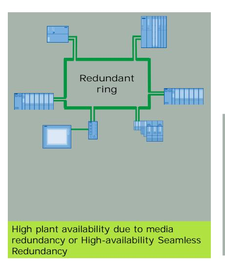
As Rapid Spanning Tree Protocol (RSTP) does not fulfill the required recovery times, several different redundancy approaches are defined in IEC 62439-series.
