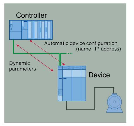
Automatic reconfiguration following device replacement without engineering and without memory card
