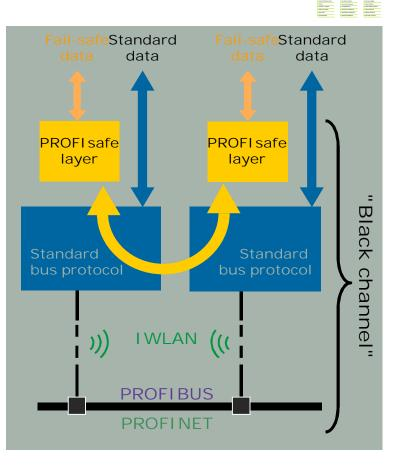
Functional safety can be used without the need of separated communication cables. Even wireless communication can be used
