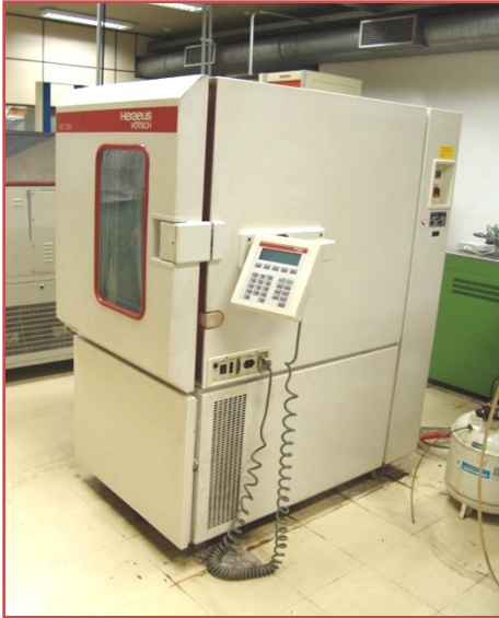
Climatic chamber – Vötsch 7033
