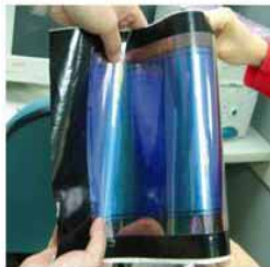
10.4" Flexible monochrome bi-stable panel
