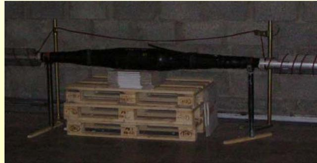
The joint was tested at  $1.45 U_0$  presented no PD at all (sensitivity: less than 5 pC)
