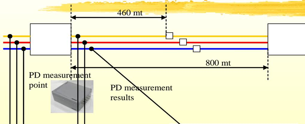
Measurements carried out from termination (short cable length)
